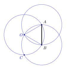
Hence, using arcs instead of full circles you could use A and B to locate O, then from B get C and continuing around the circumcircle constructing the other vertices of the regular hexagon.
